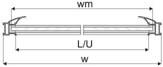
Dimensions helpful during installation of horizontal mid-rails in Simple 10 Frame systems
